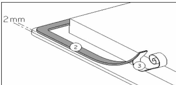
Stick the gasket (2) two millimetres from the external edge of the glass, after removing the protection sheet (3).
