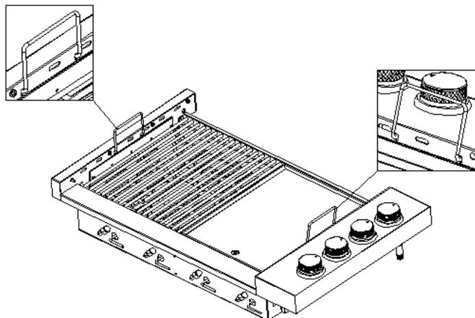
**4. Install the windshield onto the firebox.**
