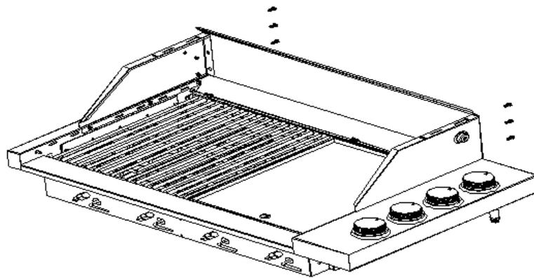
**5. Place the high lid onto the windshield and tight up. ( 2x screw type M6).**
