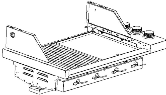
Place the backside panel ( 6x screw type M5)
